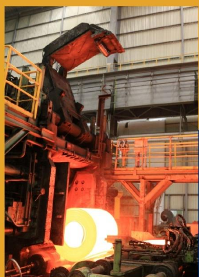
Coil Box 热卷箱 Mitsubishi-Hitachi (Japan)
